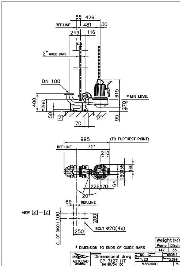
Figure 19: HT, P-installation
