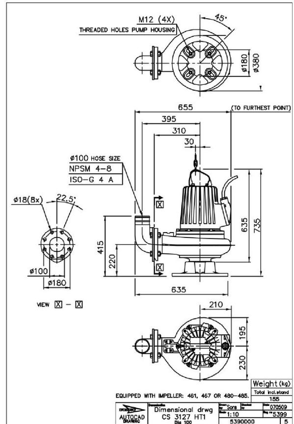
Figure 21: HT, S-installation
